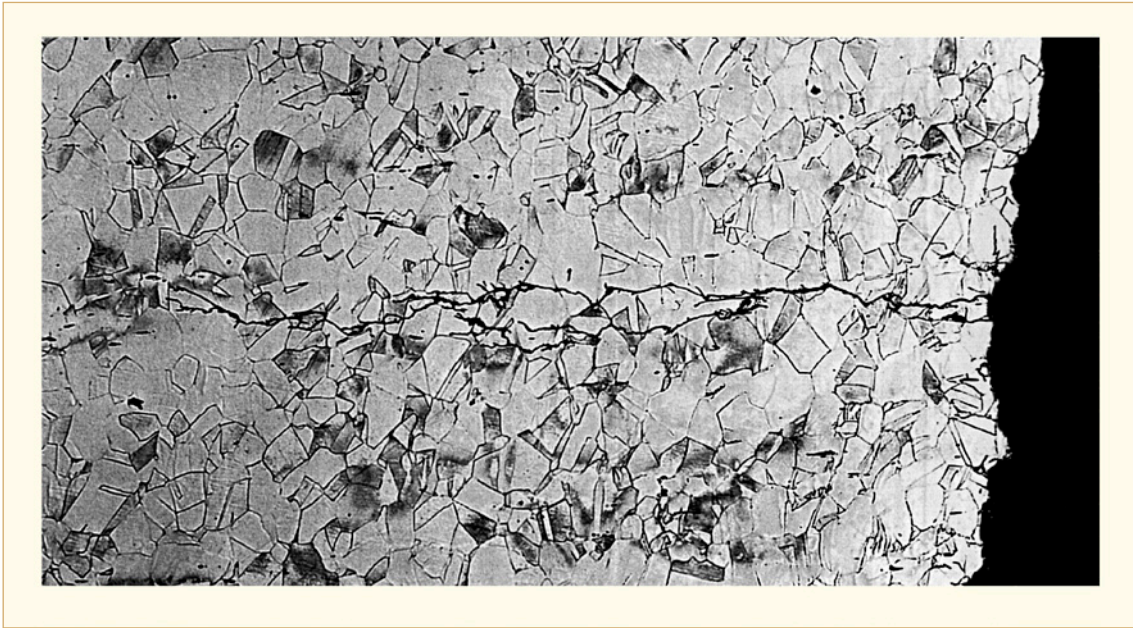
Figure 2-4: Cross section of a typical TransGranular Stress Corrosion Cracking (TGSCC) crack, SS, x48, [Boursier et al, 2002].
