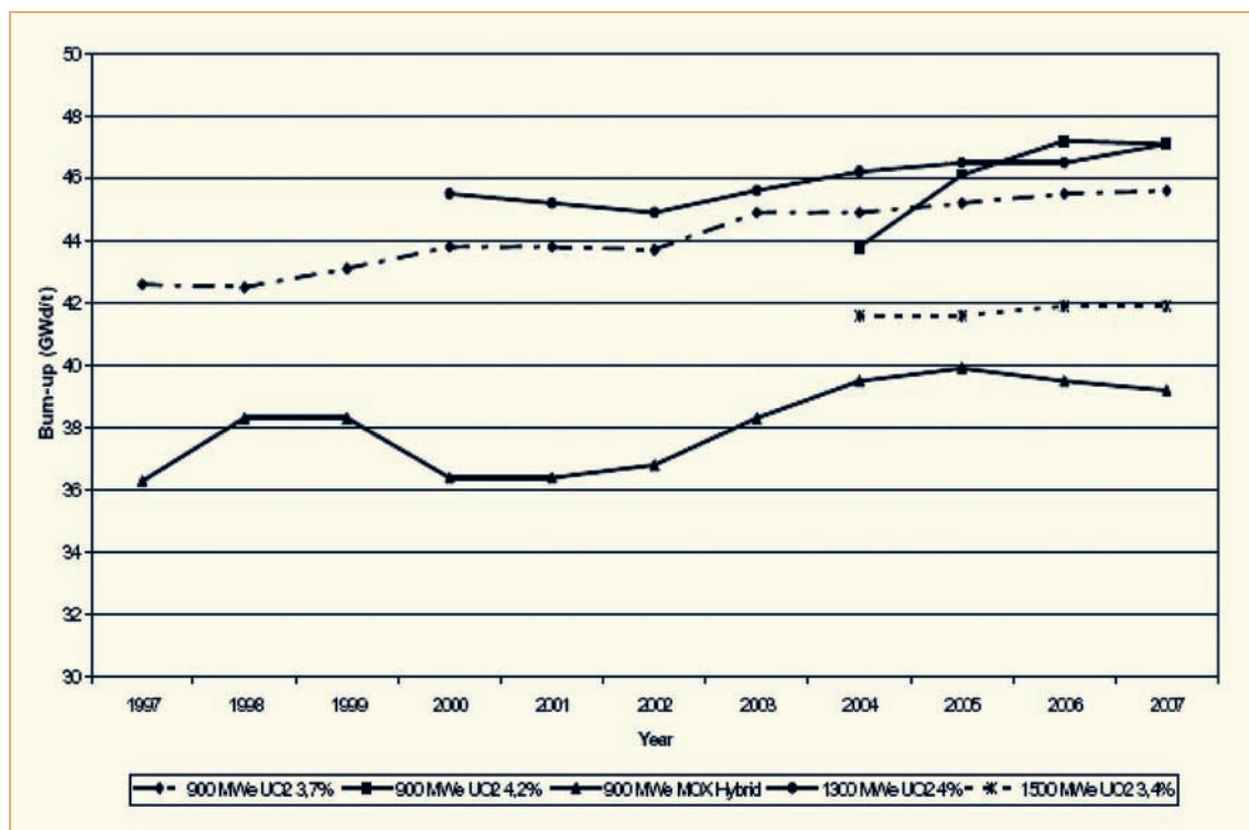
Figure 2-1: Assembly average discharge burnup trends in France, [Thibault et al 2009].
