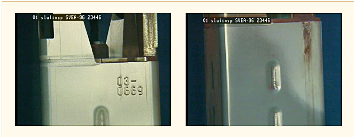
Figure 2-2: Photos showing normal oxidation features of fuel channels. The figure to the right shows some Shadow Corrosion as a result of the core grid, provided by the courtesy of OKG-EON.
